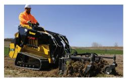
**OPTIMAL POWER.** Equipped with a 40-hp (29.8-kW) turbocharged Kohler KDI diesel engine. This engine eliminates the need for a diesel particulate filter (DPF), helping reduce cost and complexity of the engine.
