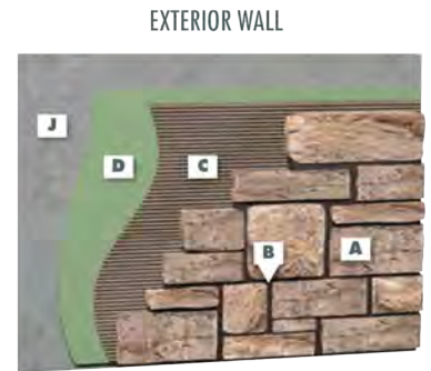
EXTERIOR WALL Concrete wall – Direct adhered with fluid applied MVIS™ Air & Water Barrier
