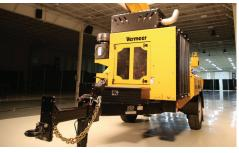
**TRANSPORT FRIENDLY.** The fully configured AX17 is under 10,000 lb (4,536 kg) helps with ease of transportation around congested urban areas and minimizes the need for additional license requirements.
