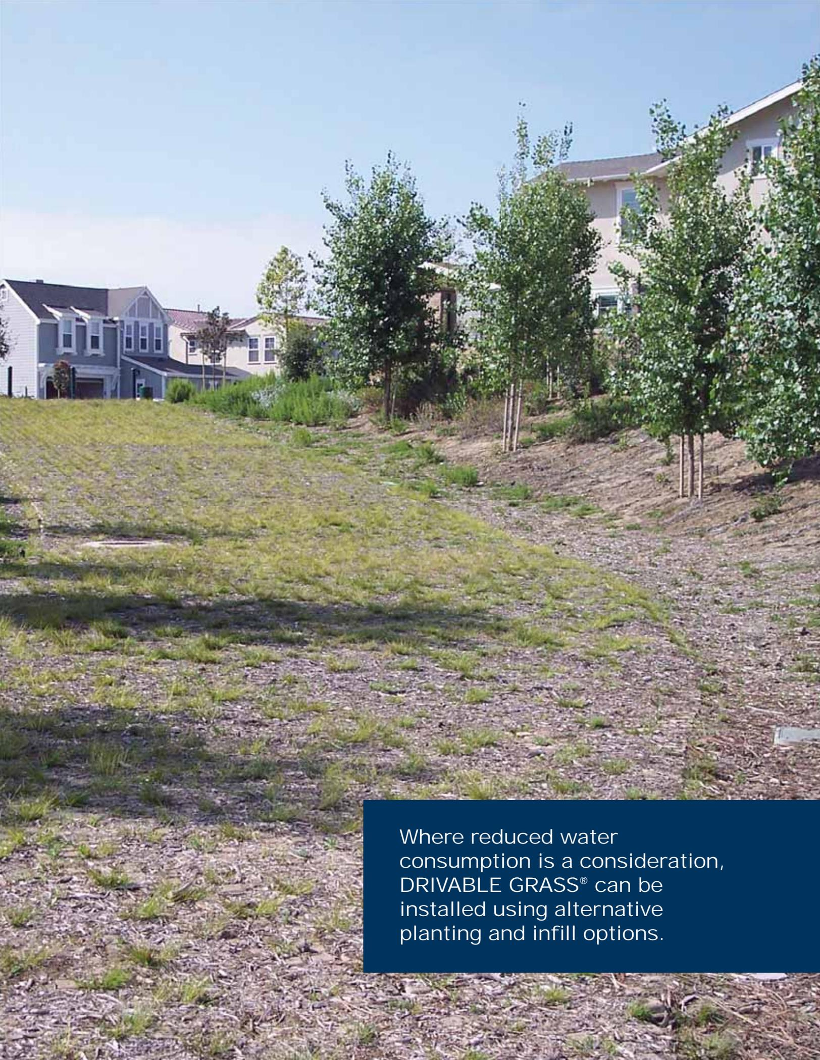
Where reduced water consumption is a consideration, DRIVABLE GRASS® can be installed using alternative planting and infill options.
